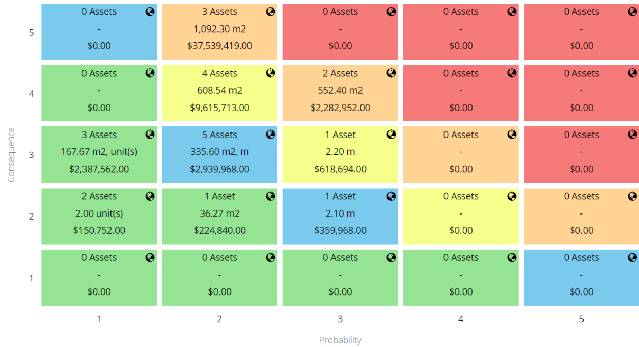
Figure 26 Risk Matrix - Bridges and Culverts
