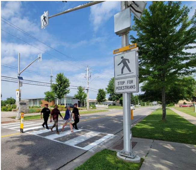
Signalized pedestrian crosswalk.
