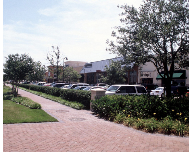
Lowered parking surfaces and landscaped buffers help screen parking areas from street view.
