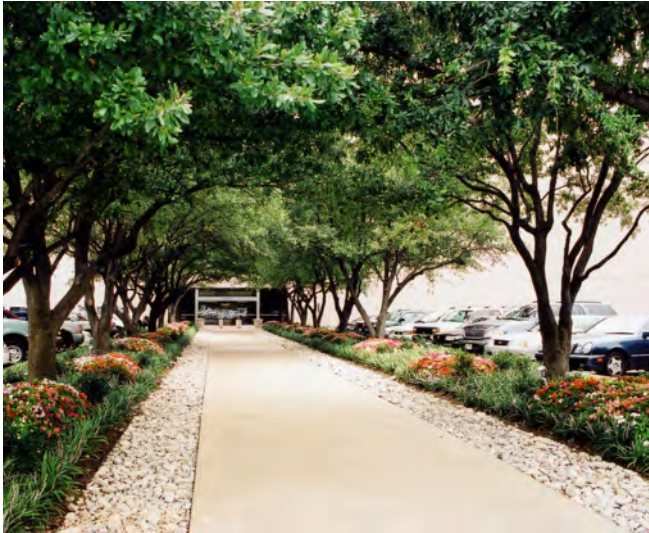
Landscaped islands, pedestrian walkways with distinct paving, lighting, and plantings provide safe crossing through the parking lot.
